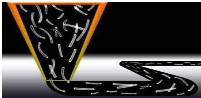
Figure. 2. The process of extrusion of 3D product manufacturing using the FDM technology from a composite material (polymer and carbon nanostructures).
