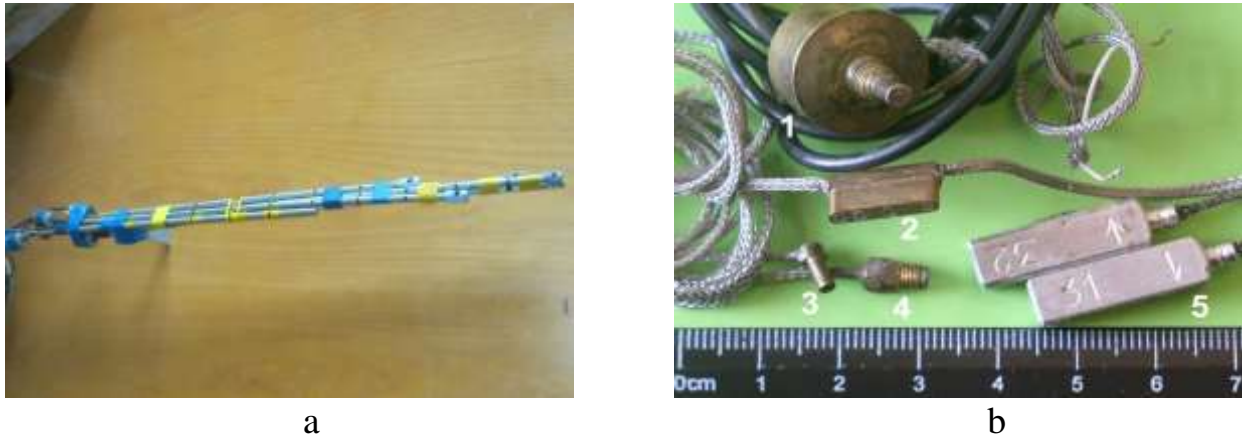
Fig. 2. Piezoresistive wave height sensors (a) and piezoceramic pressure fluctuation sensors (b)
