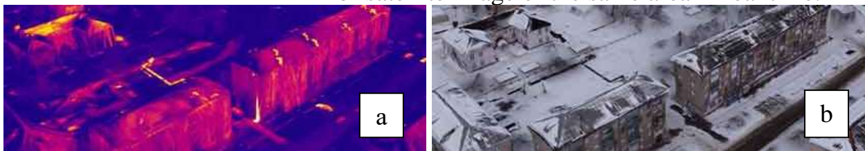
Figure. 2. Satellite images in the form of three-dimensional models: a - satellite image using a thermal imager; b - satellite image of the same area in real time.
